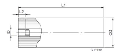
OD = outer diameter of spiral membrane
